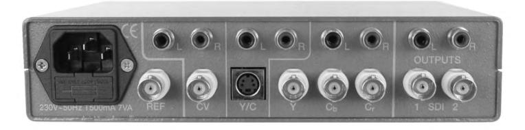
The panel plug has a fuse carrier for 5X20 fuses. In case of fuse failure, replace it with an **equivalent** one, as specified at the back of the unit.
